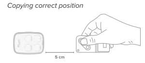
4. Nearby the gate/garage (within 5 meters) press the 1Control WHY copied button for 10+ seconds, the green LED start flashing. Wait for the LED to turn off. If the green LED does not flash, it is necessary to proceed with the guide B.
